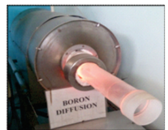
Fig.5 Diffusion process placed in boat
