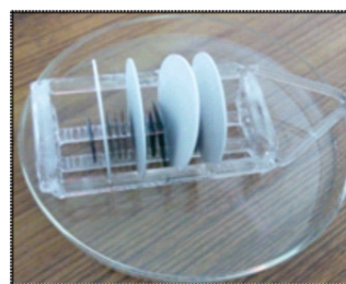
Fig.4 For Diffusion BN with wafer arrangement
