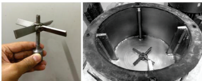
Fig.2 Bottom Propeller shaft with a PTB type propeller (b) Inside View of Slurry pot
