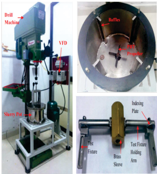
Fig.1 Photograph of (a) Slurry pot test rig, (b) Fixing arrangement of wear sample and (c) Details of Pot with PTB Propeller
