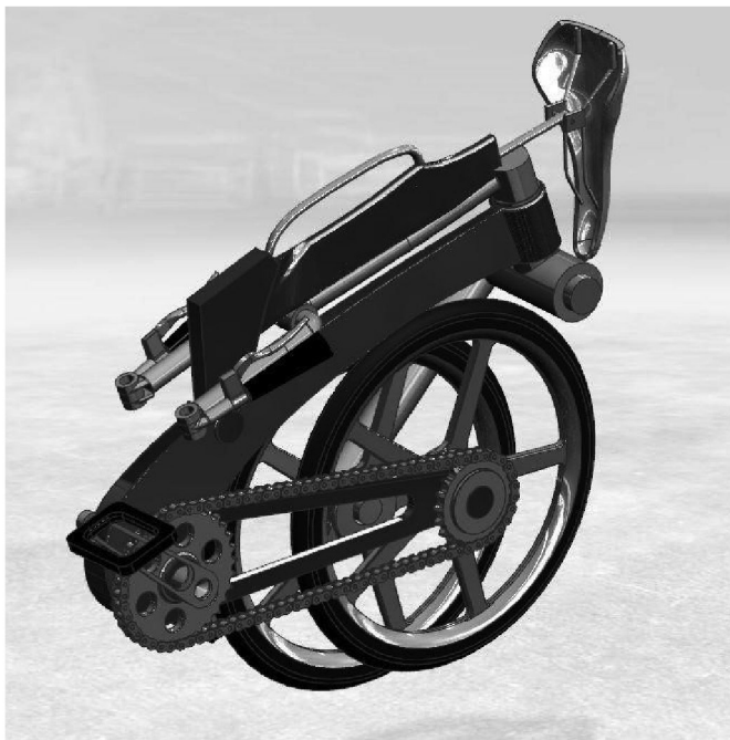
Fig.2 Electric folding bicycle in folded mode
