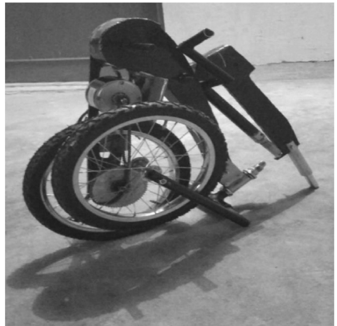
Fig.10 Assembled view of EFB after folding
