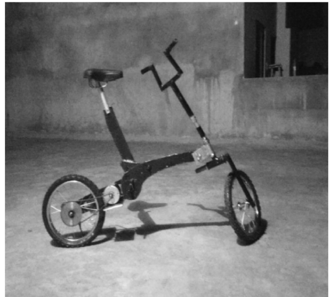
Fig.9 Assembled view of EFB in normal mode
