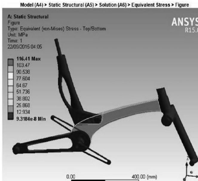
Fig.6 Maximum equivalent stress in frame2
