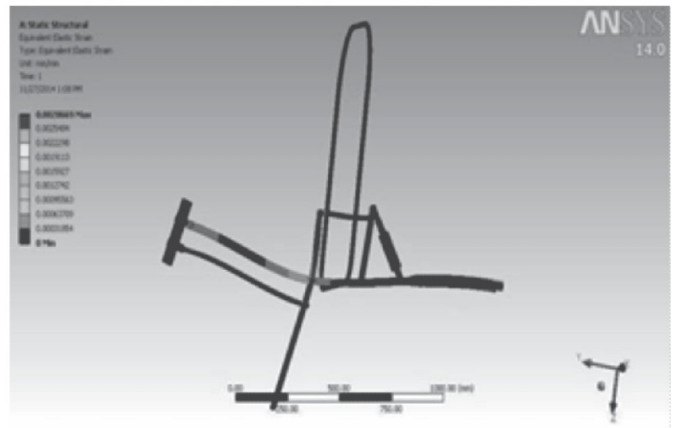
Fig 5: The equivalent stress for frame
