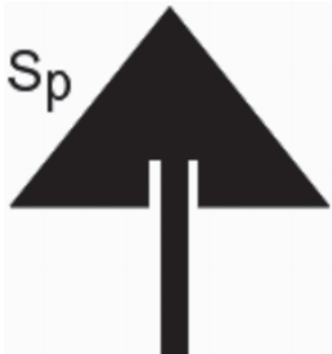
Fig 1: Equilateral triangular patch antenna with inset feeding
