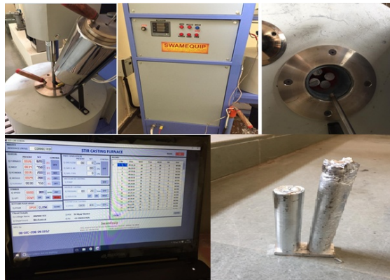
Figure 2 : Setup of stirring casting machine for fabrication of MMCs
