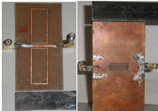
Fig. 2(a). Fabricated Dual Mode Band Reject Filter (Top Layer) (Left) (b). Fabricated Dual Mode Band Reject Filter (Ground Layer) (right)
