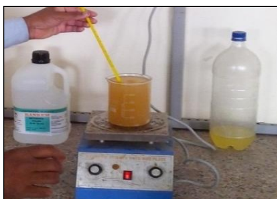
Figure 2 : Mixing of oil mixture on magnetic stirrer with heating plate.
