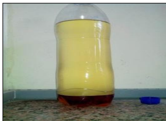
Figure 4 : Glycerin deposited in the bottom
