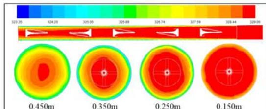
Figure 20 CFD contour for case 11
