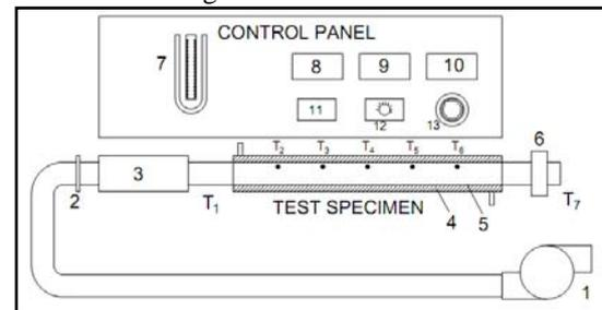
1. Blower, 2. Orifice, 3. Heater, 4. Insulation Wall, 5. Copper Tube, 6. Pressure Valve, 7. U-Tube Manometers, 8. Voltmeter, 9. Temperature, 10. Ammeter, 11. Dimmer for Blower, 12. Temperature Sensing Points 13. Voltage Controller
