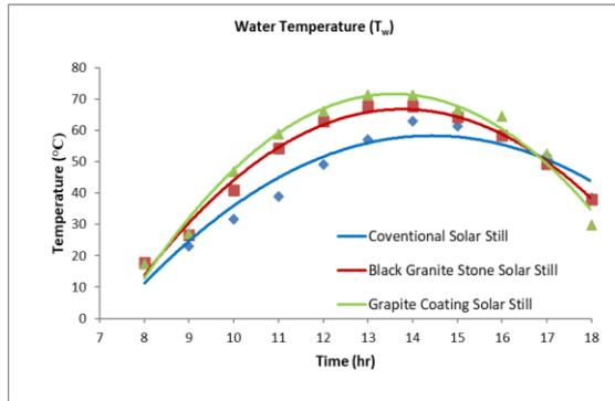
Figure 6: Variation in the basin water temperature of solar still with time of the day (March 07, 2022)
