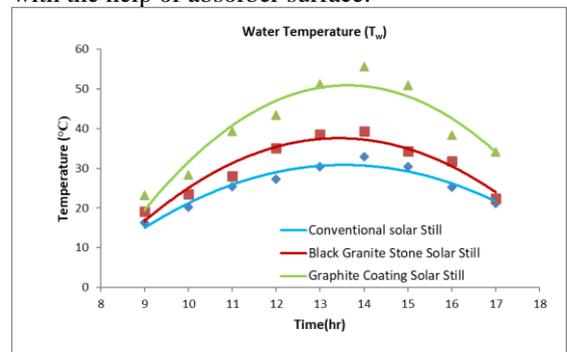
Figure 5: Variation in the basin water temperature of solar still with time of the day (Dec 23, 2021)
