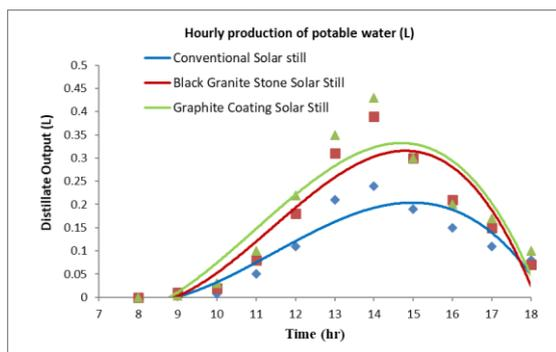
Figure 8: Hourly production of potable water with various solar stills (Mar 07, 2022)
