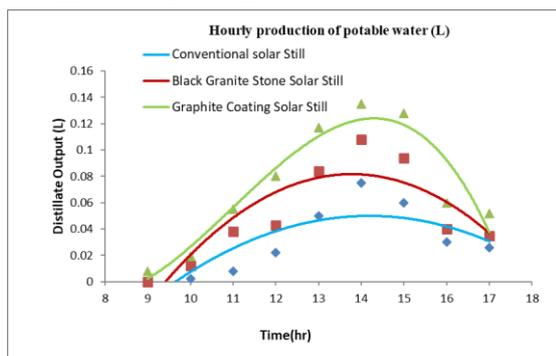
Figure 7: Hourly production of potable water with various solar stills (Dec 23, 2021)
