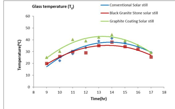
Figure 3: Variation in the temperature of glass cover with time of the day (Dec 23, 2022)
