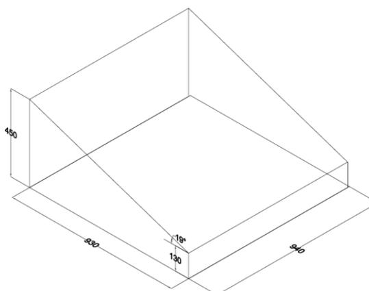
**Figure 1:** Dimension of solar still
