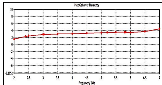
Figure 5: Variations of gain with frequency
