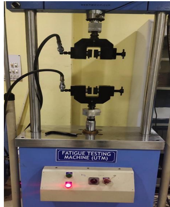
Figure 5: UTM machine used for tensile strength measurement
