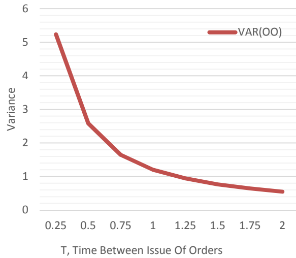
Figure 1: Change in variance of Outstanding Orders with respect to change in time between orders
