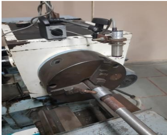
Fig.4. Setup of NPN proximity speed sensor on lathe machine
