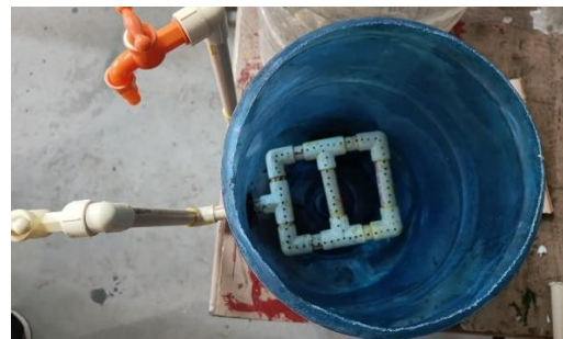
Figure 3: Lateral drain arrangement in filters
