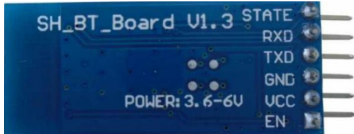
Figure 4: Bluetooth module pins
