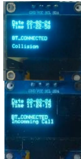
Figure 12: Result on OLED display
