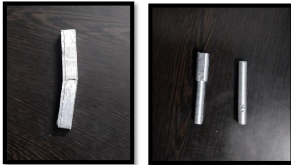
Figure 5 and 6: Shows the specimen used for tensile and flexural test after test.
