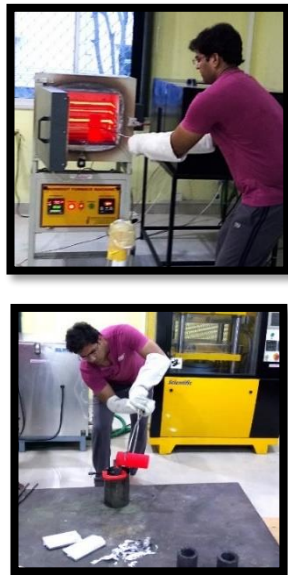
Figure 3 and 4: Melting and Pouring Molten Metal and fabricated MMCs (Courtesy: MNIT, Jaipur)
