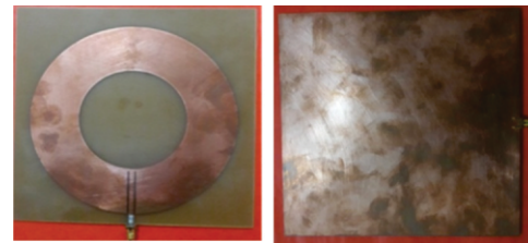
Figure 4 Fabricated Structure of the annular ring patch antenna designed by using the proposed formulae (a) front view (b) Back view.
