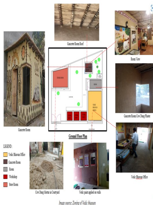
Image source: Zoning of Vedic bhavan Fig 3: Vedic bhavan made by cow dung (Monu Dalal, 2021)
