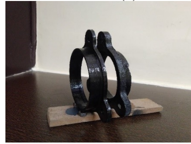
Figure 3: Flanges to hold the samples
